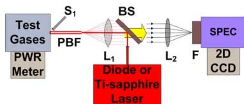
Figure 1a: L1: 11-mm aspheric singlet, L2: 6-cm efl spherical singlet, BS: dichroic long-pass beamsplitter, SPEC: 0.55-m grating spectrometer, 2D CCD: Princeton Instruments SpectruMM 250B with Hamamatsu MPP back illuminated 1024X252 element sensor array, S<sub>1</sub>: fusion-splicer cladding seal
