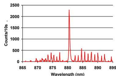
Figure 1b: Stokes spectrum of methane ( $1532 \text{ cm}^{-1}$  line). Rotational-vibration substructure is clearly visible despite the low Raman cross section. HC-800-01 PCF [2], pump power  $\sim 15 \text{ mW}$  ( $\lambda = 780 \text{ nm}$ ), ten second integration time
